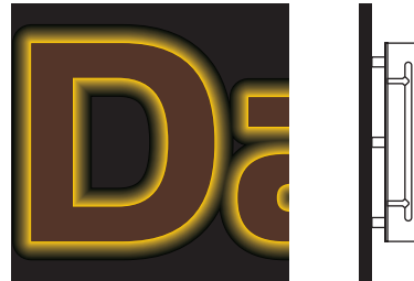
Reverse Channel "Halo" Internal Illumination
